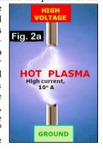
Subtle differences in *electrical breakdown* of gases differ due to: (i) Dissimilar electron-impact ionization processes in Atoms or Molecules due to Internal Energy Partition dynamics, defined by the constituent atom *Electronegativity*, *Ionization Potential etc.* (ii) At atmospheric pressure lower than normal, fewer ionizations per unit volume happen due to longer *mean-free-path*, causing insufficient
