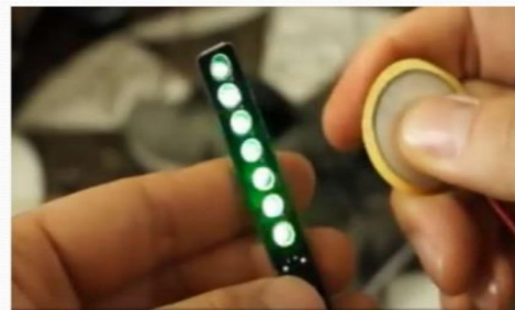
Fig. 15: Demonstration of energy harvesting with the help of piezo-transducer [61]
