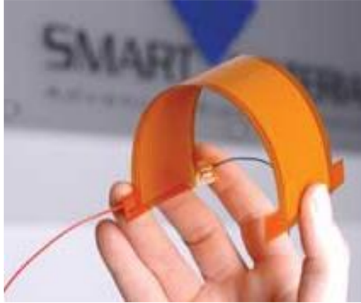
Fig. 16: Flexible Piezocomposites for energy harvesting [62]
